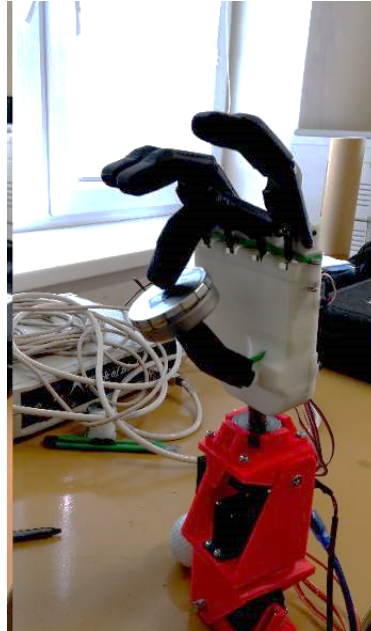
Fig. 8 Simulation of Gripping a Physical Object [4]
