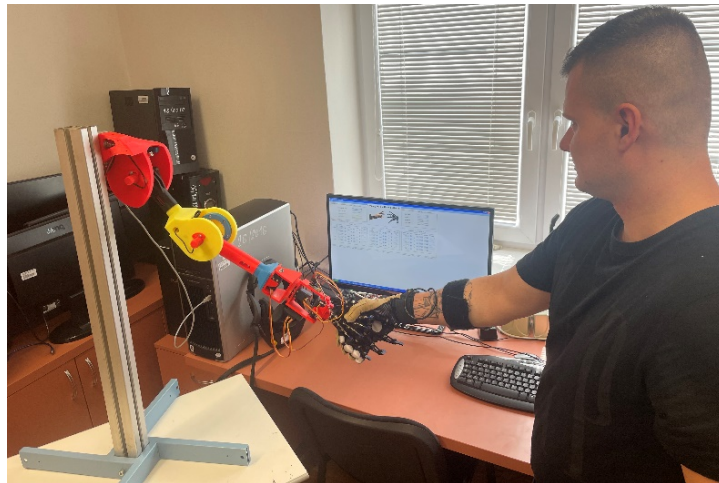
Fig. 7. Synchronization of Movements between the Data Glove and the Robotic Hand
