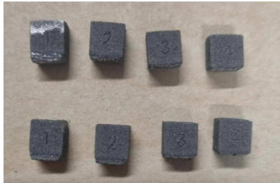
Fig. 2. 3D printed cubes using the SLM method
